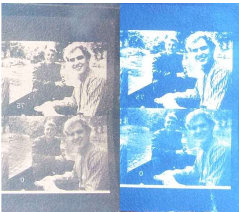
Tea toned cyanotype (left) and untoned cyanotype (right)
